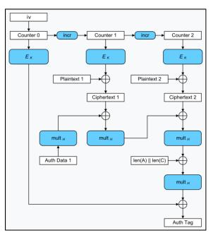
Based on the value of the initialization vector (IV), counter blocks are created. Each counter block is encrypted with the main key (e.g., AES key - operation Ek). The encrypted counter blocks form a key stream. The key stream is combined (XOR operation) with the plaintext stream, thus creating the ciphertext. It should be noted that knowing the value of the ciphertext and the plaintext value, one can obtain the key value (key = ciphertext XOR plaintext).
