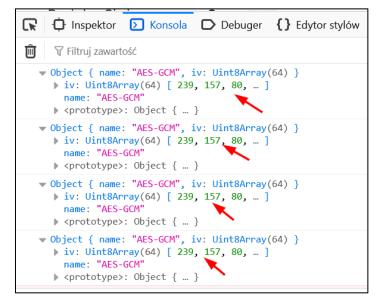
The display of the IV values used was achieved by an injection, using the Burp Suite Proxy tool, a console.log call into the application's JavaScript code performing encryption using the crypto.subtle.encrypt function:
